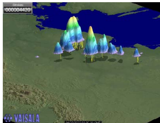
Figure 13. A thunderstorm growth and dissipation demonstration product showing VHF total lightning mapping and CG lightning activity from Poland on 4 July 2002. "Cloud-like" features represent total lightning flash rates. The higher the altitude of the "cloud-like" feature and the brighter the color (from purple to red), the higher the total lightning flash rate. CG flashes in yellow show the exact location of the CG flash on the terrain map. The area covered by total lightning is shown by a shadow-effect on the terrain map. (Patent pending)
